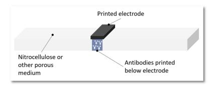
Rather than measuring the optical density of gold nanoparticles captured (or not) on the test line, we measure the change in conductivity/resistance of the current. The presence of gold will increase the flow of electrons, increasing conductivity / decreasing resistance.
